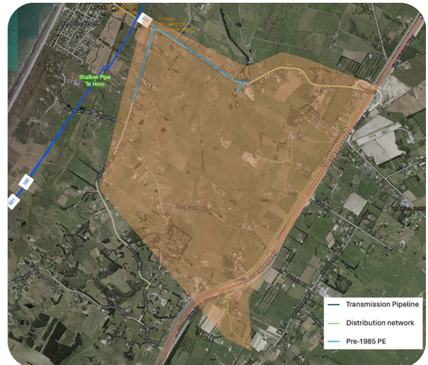
Figure 12. Network details with pre-1985 PE piping highlighted in blue.
