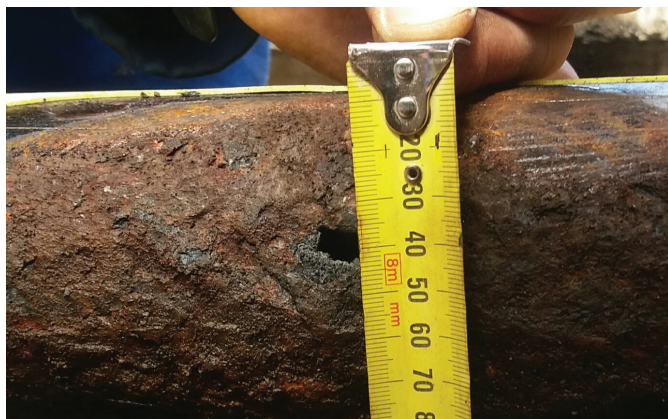
▲ One of the sections of 80NB Carbon Steel pipeline at Pukete Bridge with severe corrosion
